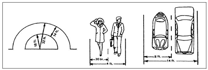
Figure 18. Minimum dimensions for access specifications.
